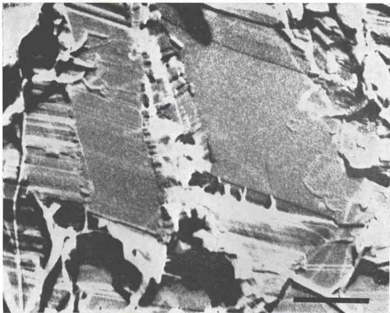
Fig. 4. Fracture surface of sample E, showing smooth fracture surface.
